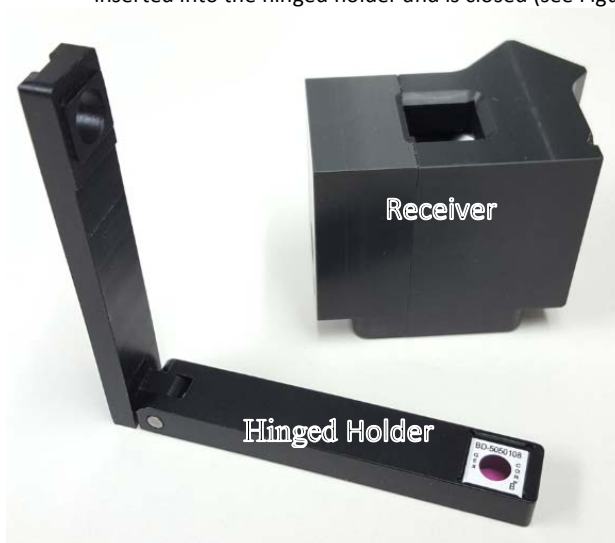
FIGURE 9: WINdose Dosimeter Holder - Receiver and hinged holder
