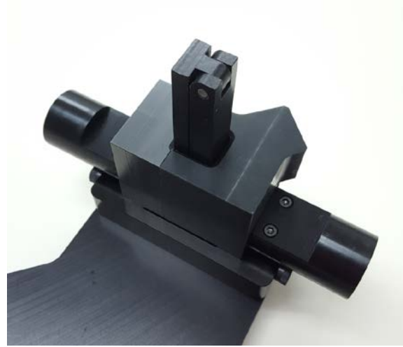
FIGURE 12: WINdose Dosimeter Holder inside receiver
