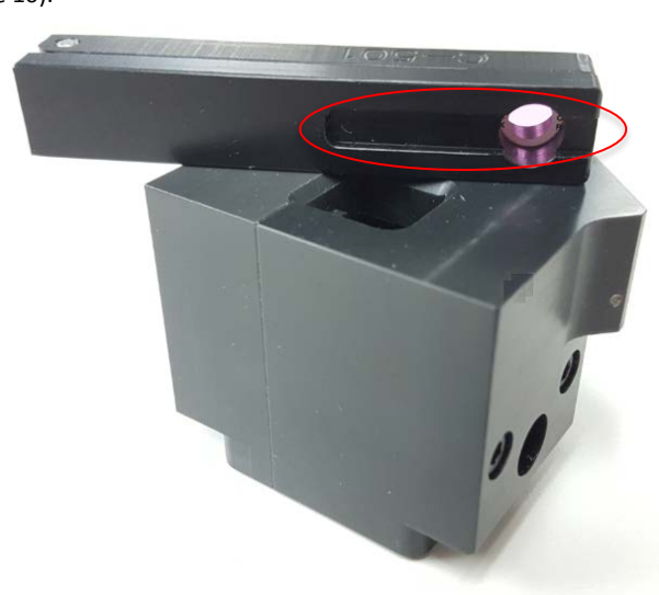
FIGURE 10: WINdose Dosimeter Holder loaded with dosimeter and featured keyed slot
