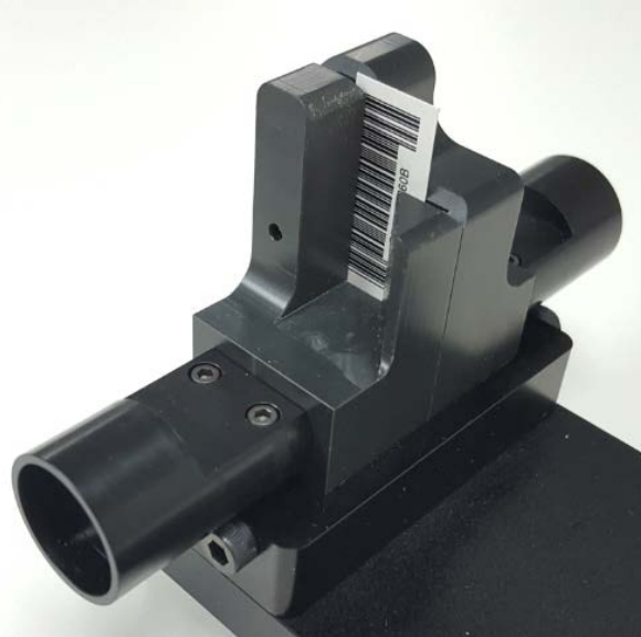
FIGURE 8: DoseStix Dosimeter Holder installation
