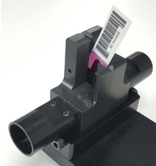
FIGURE 7: DoseStix Dosimeter Holder installation
