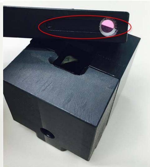
FIGURE 10: WINdose Dosimeter Holder loaded with dosimeter and featured keyed slot
