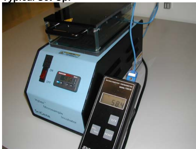
Digital Thermometer connected to Micro Incubator. Temperature agreement is 0.1°C
