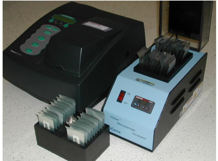
Note: Al holder block shown outside of the incubator is shown as visual aid. The aluminum block is maintained inside the main cavity of the incubator at all times and is only removed for periodic cleaning. Turn the power off when block is removed from the incubator's cavity.
